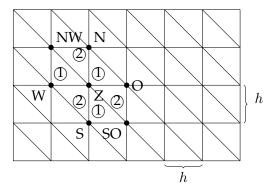
Basis functions of all inner nodes look the same and therefore all rows of the stiffness matrix are identical (except for boundary nodes). As a consequence it is sufficient to look at only one node Z. Let N, O, SO, S, W, NW denote the neighbours of Z.
