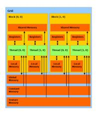
Memory hierarchy with specific access of individal instances (thread, block and grid)
