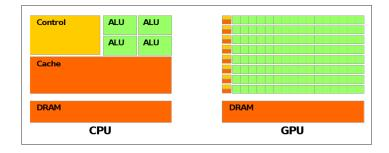
GPU tremendously more transistors for data processing, therefore fewer transistors for cache
